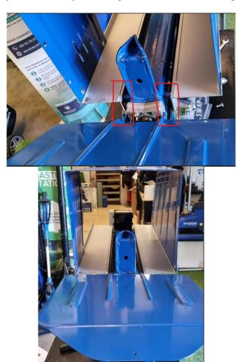
Position the side plastic protections by inserting the 10 fixing clips by force
