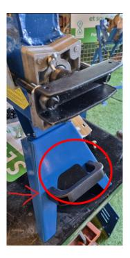
• Screw the 2 side plates together with 4 brackets and 4 nuts, bolts and washers
