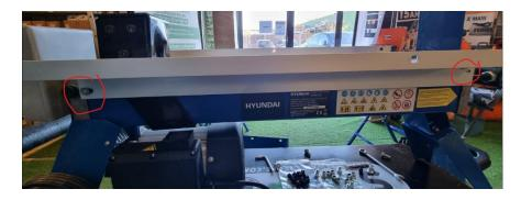
• Screw the side protections with 6 nuts and bolts and 3 nuts, bolts and washers as below:
